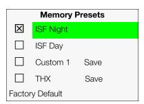
For each input, the VX-33d lets you save image quality settings as presets that you can recall at a later time. You can create up to four presets per input and resolution. Use the ISF Presets menu to recall saved image presets, or to save image settings in the "Custom 1" or "THX" memory location. The currently-selected preset is indicated by a "\overline{\text{\text{M}}}" to its left; in the example shown here, ISF Night is selected.
